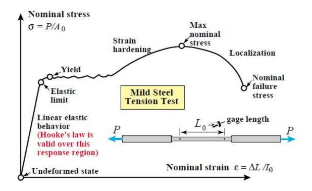
**Figure 1.4:** A typical tension test behaviour of mild steel with well defined yield point and extensive yield region.
