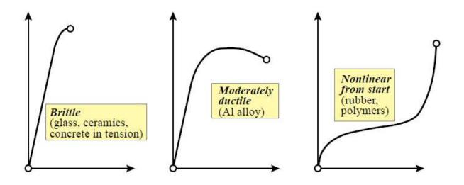
Figure 1.5: Three material responses during tension test
