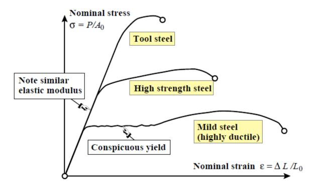
Figure 1.6: Response of three grades of steel to loads
