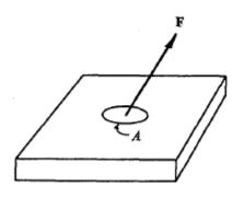
Figure 1.2a: Normal stress component  $(\sigma)$
