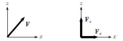
Figure 1.0: Resultant force and the components of force.
